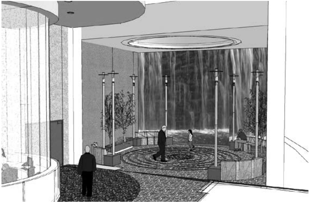
Figure 2-3. Proposed water feature for the ER One Project at Washington Hospital Center, Washington, DC. This feature is planned to mitigate stress as a positive distraction. In addition the water wall also acts as “blast” protection from outside forces. ILLUSTRATION: Patricia Raimondeau
